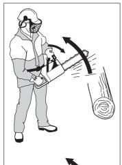
If the kickback is less violent or the kickback zone of the bar is closer to you the chain brake will be activated manually by the movement of your left hand
